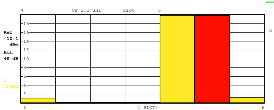
Fig. 5-11 Composite EVM diagram with unrecognized channels
